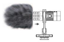
4.Connect the 3.5mm output jack of S20 with the 3.5mm input jack of DSLR camera via the 3.5mm TRS cable.
