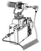
5.For the professional stereo effects, please connect a extra microphone like the customized lavalier microphone to the \$20 and toggling the mode switch button to "S" mode. In this manner, you can obtain a stereo sound which is more suitable for interview purpose.
