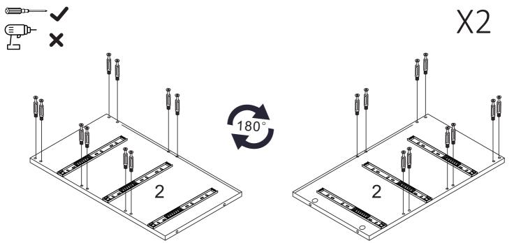
I.Attach panel (4,5,6,6,6) to panel (3),insert cam-lock (B) into the panel (4,5,6,6,6), then turn clockwise to lock onto cam-bolt.
