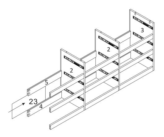
I.Attach panel (1) to panel (4,5,6,6,6,23), insert cam-lock (B) into the panel (4,5,6,6,6), then turn clockwise to lock onto cam-bolt.
