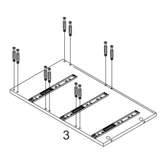
I.Use screws (C) to secure the slide rail (E1) to the panel (2), and tighten them with a screwdriver.
