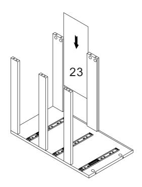
I.Attach panel (2) to panel (4,5,6,6,6,23),insert cam-lock (B) into the panel (4,5,6,6,6), then turn clockwise to lock onto cam-bolt .
