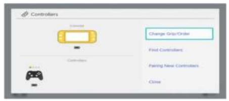
4). Click "change grip/order" to enter the pairing interface. Press and hold Docking button for 3 seconds to establish pairing, 4 LED indicators flash, release your hand, wait for 5-30 seconds until pairing succeeds and controller icon shows up on the screen, corresponding channel LED indicator keeps on.
