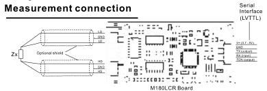
When power supply is applied, the LED on M180 board will quick blink twice and then blinks in about 1Hz, indicating the board is in normal working state.
