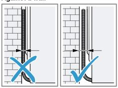
Do not trap the hoses and power cord between the wall and the appliance.
