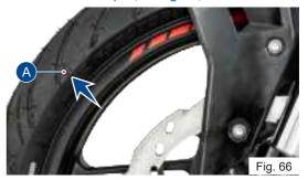
Tread depth of the tyre should be minimum 2 mm if the vehicle speed is higher than 100 km/h, and it shall be minimum 1 mm if the vehicle speed is
