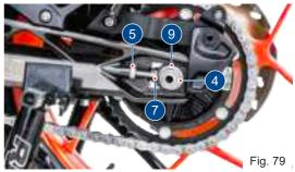
Remove the chain tensioner and push the quickrelease axle (10) to the right as much as possible (ref. Fig 80).
