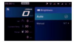
By setting display in auto mode, the connected instrument TFT cluster's intensity adjusts automatically based on the ambient light sensor.
