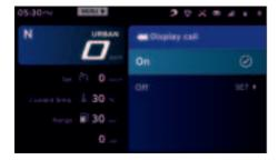
If the display call setting is turned 'ON', the connected TFT instrument cluster will display the incoming call alert from the smart phone via Bluetooth. For example call from 'Vivek' will be displayed as shown below if the contact is stored in the smart phone otherwise the number will be displayed.
