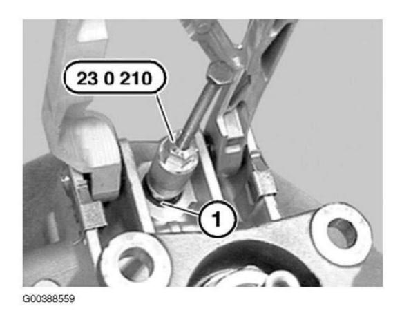
Fig. 11: Pulling Out Radial Seal For Selector Shaft Courtesy of BMW OF NORTH AMERICA, INC.
