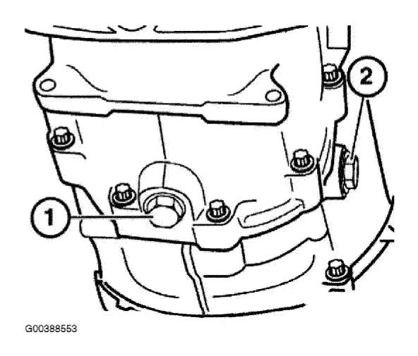
Fig. 1: Locating Oil Drain Plug & Filler Plug Courtesy of BMW OF NORTH AMERICA, INC.
