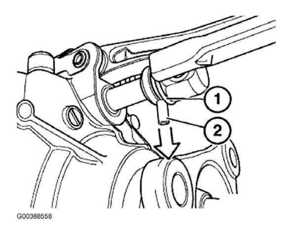
Fig. 10: Removing Retaining Ring Courtesy of BMW OF NORTH AMERICA, INC.
