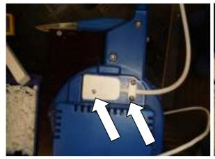
Remove the cover and the connectors as indicated by the arrows in the image above.
