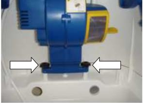
Loosen the two knobs as indicated by the arrows in the image and pull out the fan housing.
