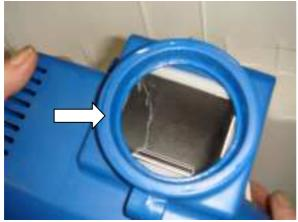
Install the gasket in the 12 V housing as shown in the image above.
