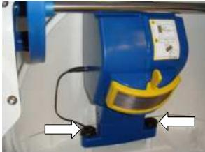
Install the fan housing using the 2 knobs and also the 2 washers underneath the fan housing as shown in the image above.
