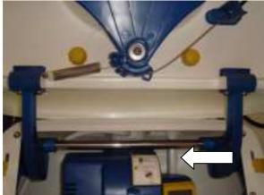
Push the plastic sleeve up through the hole as shown in the image above.
