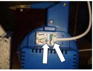
Loosen the cable as indicated by the arrows and the image above, and remove the cord.
