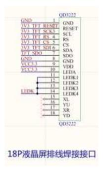
QD3222 is a 18P pad with a spacing of 0.8mm. Used to weld the LCD so that it can receive signals from the main control.
