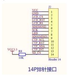
J2 is 14P pin, R8 is the pull-up resistor of SD card CS pin. The 14P pin is used to connect to the main control, which can be directly inserted or connected through a DuPont cable. Because the SD card and LCD share the SPI bus, first pull up the CS pin of the SD card to disable its functions and avoid SPI bus device conflicts when the module is in use.
