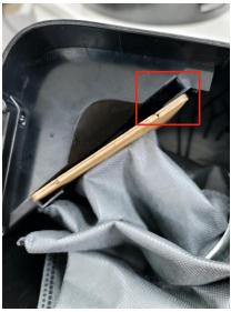
Install or adjust the dust bag as shown in the following image, close the Self-Empty Station cover, and then press the automatic dust collection icon on the app.
