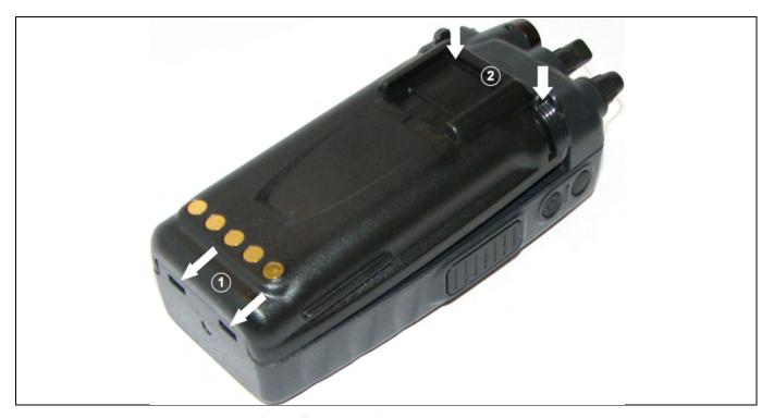
Figure 5-2: Attaching the Battery Pack
