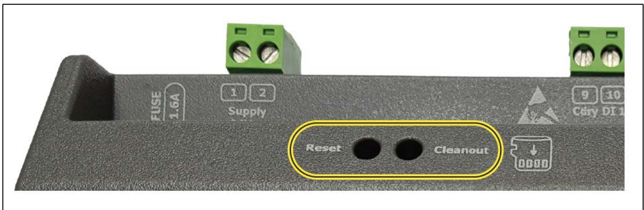
Site Supervisor Reset and Cleanout
