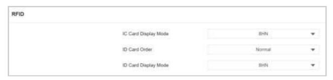
• IC/ID Card Display Mode: Set the card number format from the provided options. The default format in the device is 8HN.
