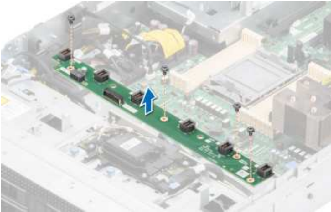
Figure 104. Removing the cooling fan cage board.
