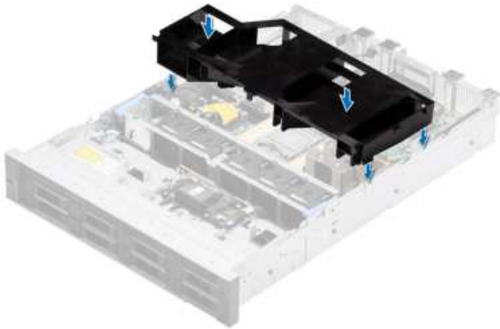
Figure 25. Installing the air shroud
