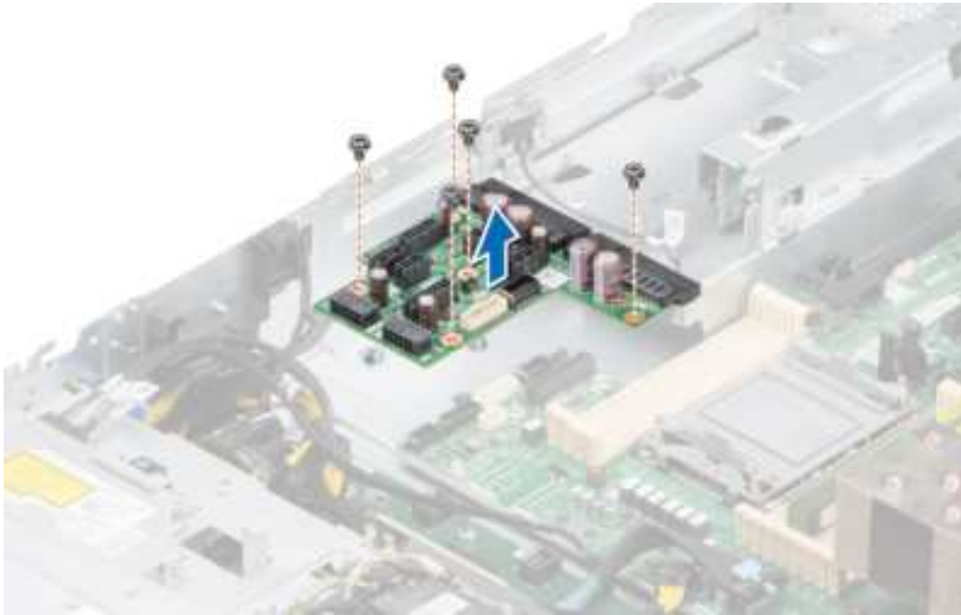
Figure 102. Removing the power interposer board
