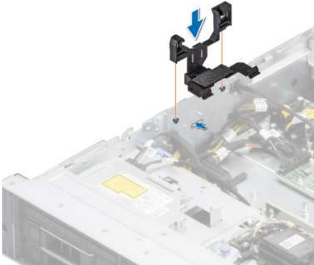
Figure 31. Installing the side wall bracket
