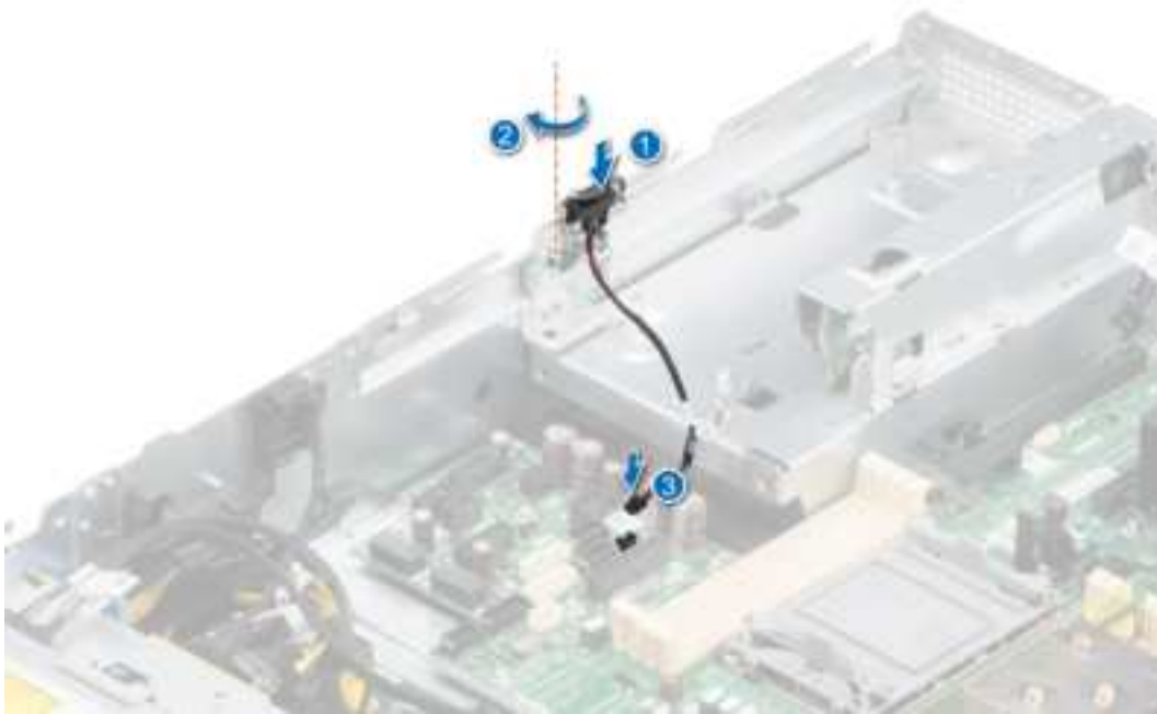
Figure 33. Installing the intrusion switch
