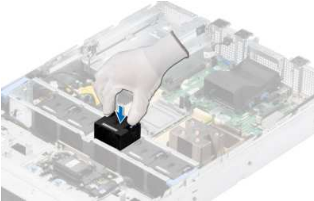
Figure 29. Installing a cooling fan
