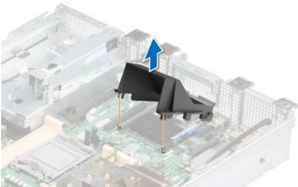
Figure 88. Removing the OCP shroud
