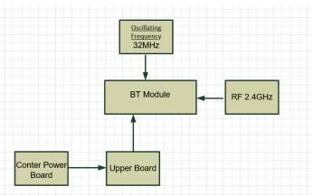
1.3 The Conter Power Board provides power to the Upper Board, which supplies power to the BT Module
