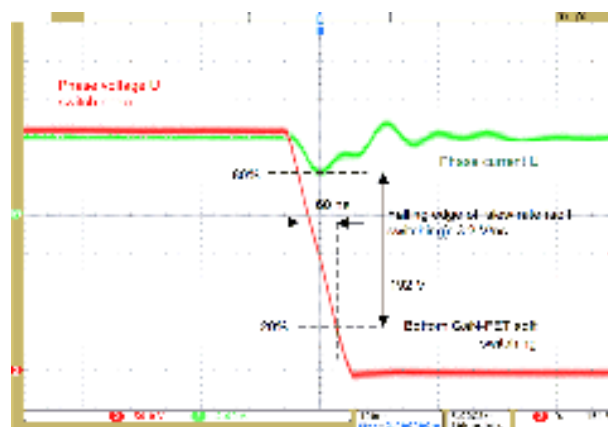
Figure 4-12. Phase U Falling Edge Waveform at 4 A, 1-m Cable to AC Induction Motor
