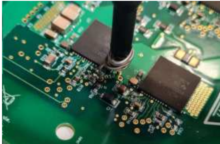
Figure 4-6. LMG3422 Switch Node Phase Voltage Measurement
