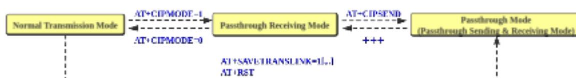
Fig. 1: Transmission Mode Shift Diagram
