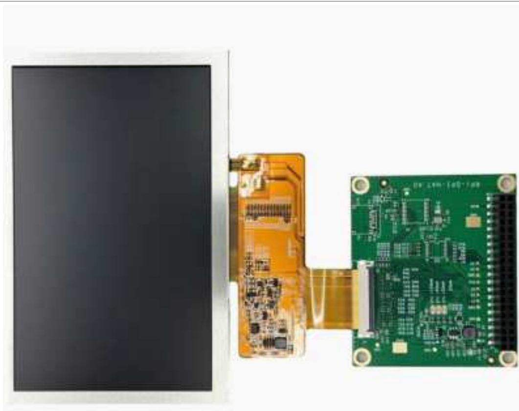
Figure 11. FPC connection between 5-inch Tianma LCD panel and adapter board
