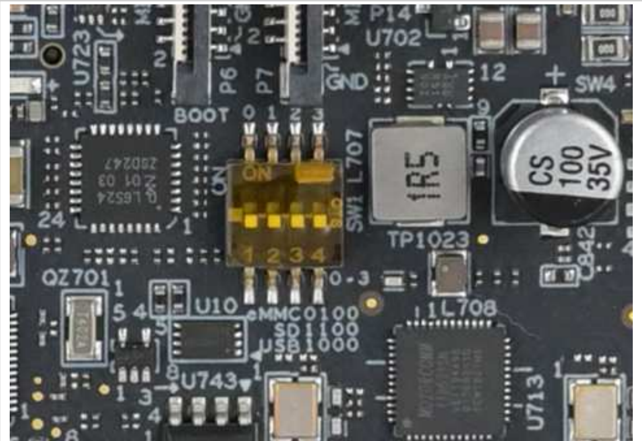
Figure 7. Boot mode selection switch
