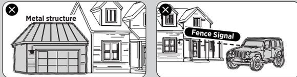
Do not attach to or near metal buildings. If there is a metal building or object in the Fence, the Fence signal may weaken in that area.
