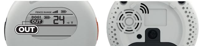
When a dog wearing the SMART FENCE collar goes out of bounds, an audible warning will sound from the Control Station. There is a two-tier alert system: one when the dog is at the boundary and another when the dog crosses it.
