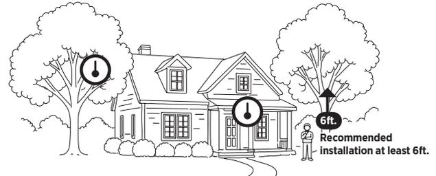
Use the provided wall mount and charging cable to install the Control Station as high as possible in order for the fence signal to emit over any objects.
