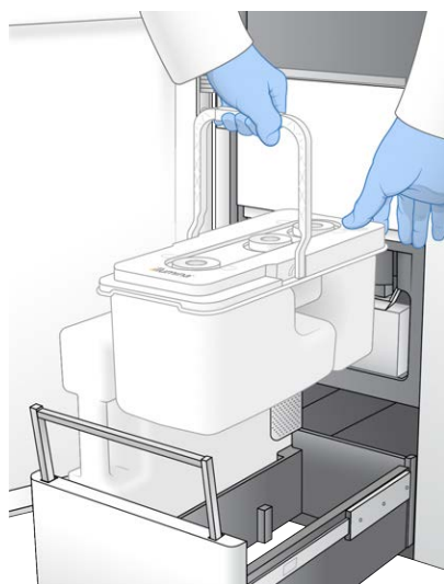
Figure 26 Load the Buffer Cartridge
