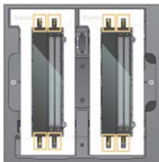
Figure 17 Loaded Flow Cells Aligned Over Clamps
