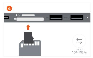
Insert micro/SD cards into adapter's card reader slots. Cards can be read simultaneously. Supports UHS-I read/write speeds.
