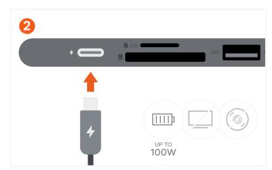
Connect USB-C charging cable to the adapter's USB-C PD charging port - up to 100W (15W used for operation). Does not support video output.
