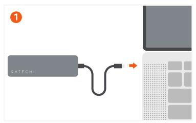
Connect the adapter to a compatible host device. LED indicator would turn on once connected.
