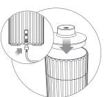
Put the lid back on, then connect the Diffuser with the USB Type-C cable to a USB plug to power on.
