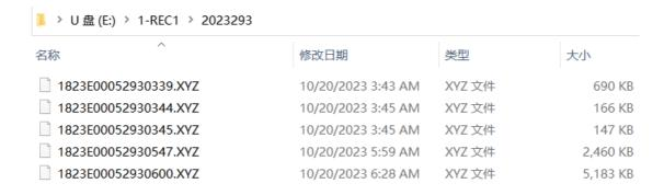
In addition, you can download the static data via WebUI, connect the WiFi of the X1 receiver and log in **192.168.10.12** (Username: **admin**, Passwords: **admin**) Go to **Work management** >> **File Download** to download the static data.
