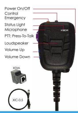
**Power Off/On:** Hold for about 2 seconds to turn on or off. The Power Mic will sound escalating or de-escalating tones to advise status. The device does a self check and the status light then glows. (see Control)
