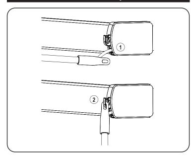
On Honeycomb shades, the wand will be already connected to the shade (1). With the wand control buttons facing you, attach the top of the wand into the plastic hook support on the motor control side (2).
