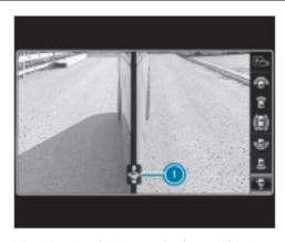
When the electrical connection is established between the vehicle and the trailer, the display changes to side camera view ①.
