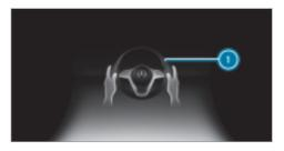
If the system detects that the driver has not steered the vehicle for a considerable period of time or has removed their hands from the steering wheel, display 1 appears in the multifunction display. If the driver still does not steer the vehicle, or gives no confirmation to the system, a warning tone sounds in addition to the visual warning message.
