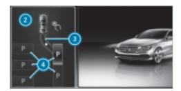
The media display shows the view of Active Parking Assist. Area 2 displays detected parking spaces (4) and vehicle path (3).
