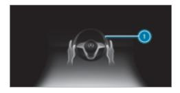
If the system detects that the driver has not steered the vehicle for a considerable period of time or has removed their hands from the steering wheel, display 1 appears. If the driver still does not steer the vehicle, a warning tone sounds in addition to the visual warning message.
