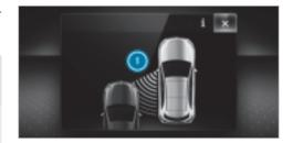
If a course-correcting brake application occurs, the red warning lamp flashes in the outside mirror and a warning tone sounds. In addition, a display indicating the danger of a side collision appears in the multifunction display.
