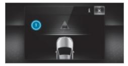
If autonomous braking or situation-dependent braking assistance has occurred, display 1 appears in the multifunction display and then automatically goes out after a short time.
