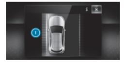
If a lane-correcting brake application occurs, display **1** appears in the multifunction display.
