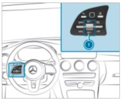
To operate cruise control or the variable limiter: press the rocker switch on the steering wheel control unit up or down to the desired position.
