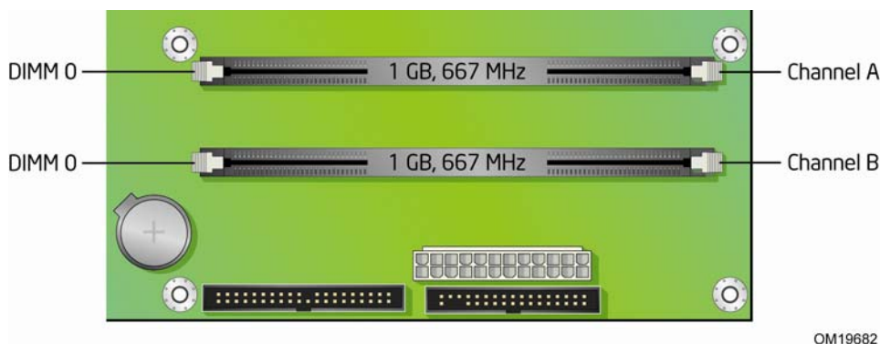
Figure 13. Dual Channel Memory Configuration Example
