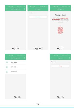
Enter to modify the fingerprint name (Fig. 19), after inputting the fingerprint name, click "Modify", the modification is successful.
