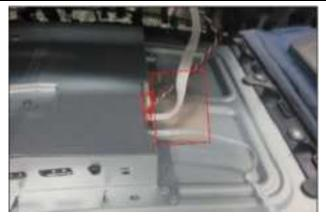
Tear off 2pcs conductive tape, release the wires and speakers. Remove the screw \* 3pcs
