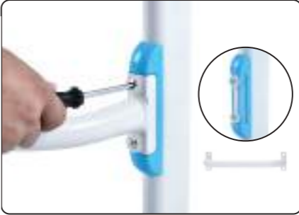
5. Remove the screws of chair leg with a screwdriver. And then take out the chair-leg connector, fit it with the chair legs together, and install the screws with a screwdriver.
