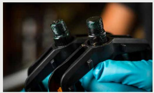
**c.** Finally, lightly grease the pedal threads.
