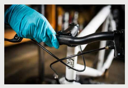
**d.** Finally, using your 4mm Allen Key, loosely tighten the stem's faceplate so that it gently holds the handlebar in place. (make sure the handlebar is centered evenly across the stem. We will fully tighten the handlebar later).
