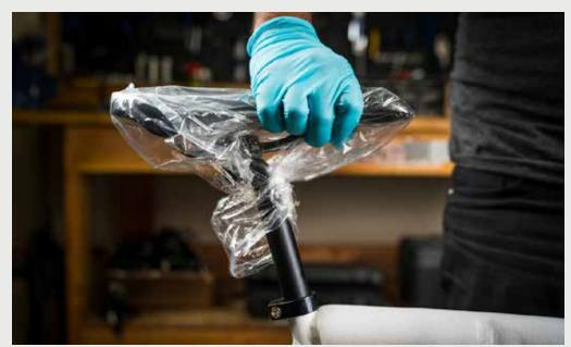
**d.** Finally, tighten the seatpost clamp with your 5mm Allen Key.
