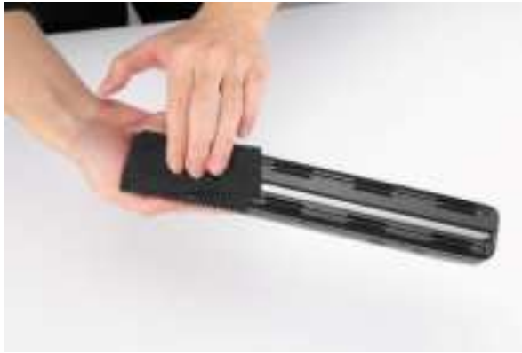
Figure 3- 1 Clean The CIS
