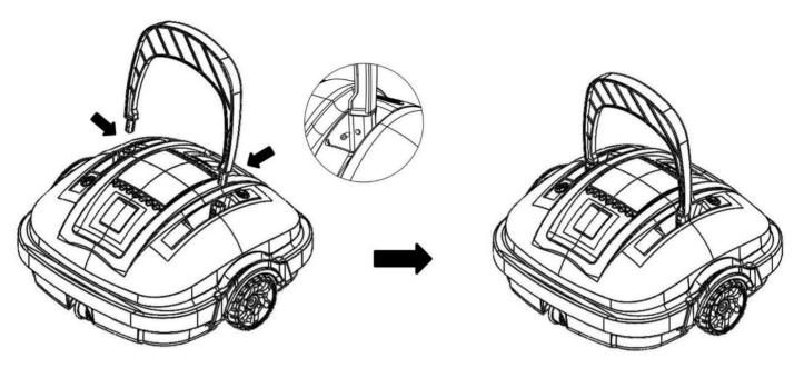
Note: The installation direction of 2 screws is opposite.
