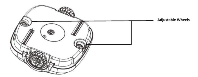
2. To adjust the wheel, open the lock buckles and remove the top cover. Locate the 2 adjustable wheels. Detach the wheel by pushing the wheel stem catch. Select the correct combination and insert the wheel until the catch clicks.
