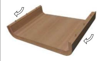
**1.3:** Place 2 staples in the slots to secure the floor panel with the lower corner panels.
