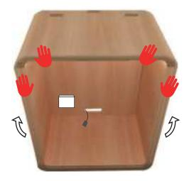
**Step 8**Set in place the last 4 staples in the union of the walls with the corners.
