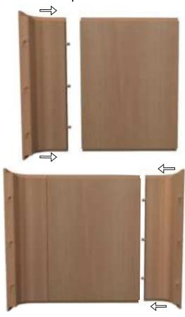
**1.1:** Place 2 staples in the slots to secure the floor panel with the lower corner panels.
