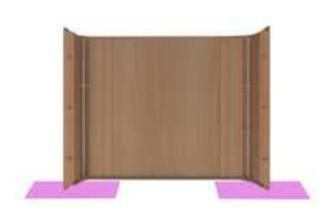
**4.1:** Fit the left wall to the base (the position is labeled on the piece).
