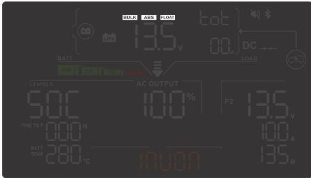
Charging Stage: Displays the active charge state: BULK, ABSORPTION or FLOAT.
