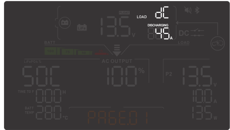
DC Discharging: The display shows the total DC current being drawn from the DC load output terminal.
