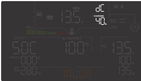
DC Charging: The display shows the total DC current provided by the PowerBoss from a DC charging input.
