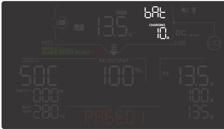
Total System DC Amps: The display shows the real-time battery current. Charging indicates that the PowerBoss is charging the auxiliary battery. Discharging indicates the PowerBoss is drawing power from the auxiliary battery.
