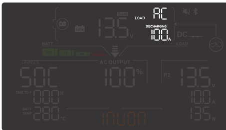
AC Discharging: The display shows the total DC current used by the inverter.
