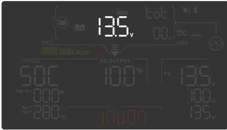
Battery Voltage: Displays the voltage of the auxiliary battery connected to the PowerBoss.
