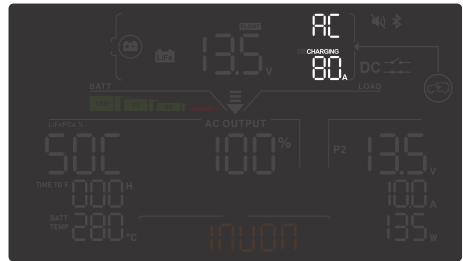
AC Charging: The display shows the total DC current provided by the PowerBoss from the AC charging input.
