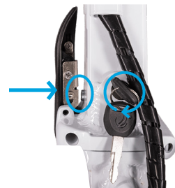
Locking Pin protruding through frame
