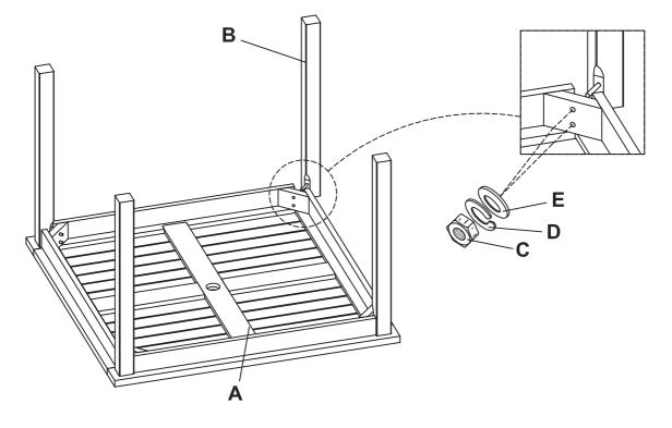
Attach the leg frame (B) into each corner of the top table (A). insert Washer (E), Spring washer (D), and Nut (C) to each leg (B). Tighten nuts using wrench.
