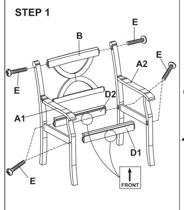
Attach the back supprot (B), front apron (D1) and back apron (D2) into side frame (A1&A2), secure using 1 1/2" bolts (E).
