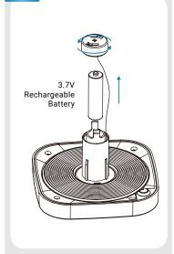
Note: To replace the rechargeable battery, unscrew the cap from the light and replace the battery.
