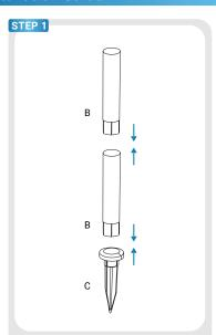
a. Remove accessories from packaging.b. Connect the light poles (B) and the ground stake (C).
