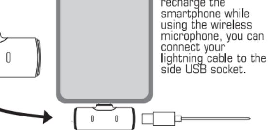
If you wish to recharge the smartphone while using the wireless microphone, you can connect your lightning cable to the side USB socket.
