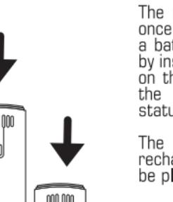
The microphone are automatically recharged once placed into the case. The case, containing a battery, needs to be periodically recharged by inserting a USB type C cable into the socket on the bottom. Each time you open the case the leds will indicate the battery charging status.
