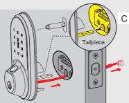
Secure the mounting plate with the supplied screws. Do not overtighten screws.
