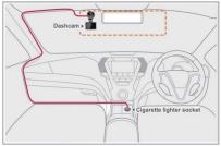
4. Plug one end of the supplied car charger into your vehicle's accessory port and the other end into the Mini-USB port on the dash cam. Route the cable alongside the interior trim of your vehicle for a cleaner install.
