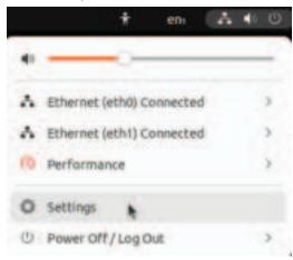
13. Toggle the Ethernet (eth0) network port to the OFF position.
