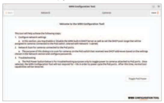
5. Enable the DHCP server for PoE Ports and provide the Start and End IP addresses. In this case we will use 192.168.55 as the subnet
