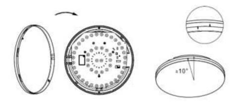
Twist the cover clockwise to fit and align the protrusions of the cover and the housing.
