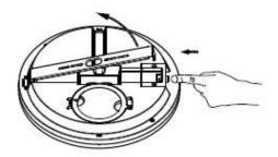
${\bf 3.}\ \ {\bf Twist\ terminal\ block\ cover\ anticlockwise\ and\ pull\ to\ remove\ it.}$
