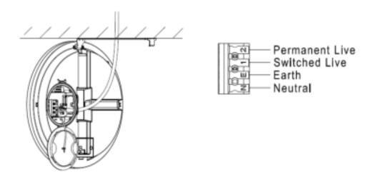
Refit the power cover (twist clockwise to secure and secure with screw.
