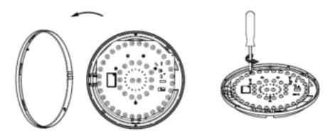
Fill in the battery installation date, and connect the battery cable (disconnected for storage) then replace the light source PCB back to original position and secure the screws. (24 hour charge time required)
