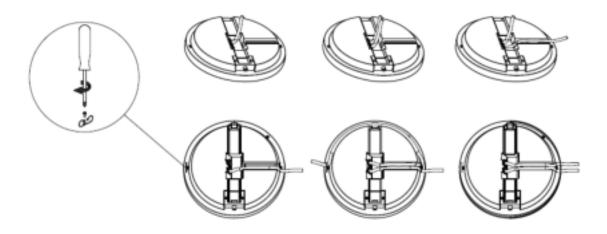
8. Connect the mains switched live, permanent live (if present) and neutral to the push terminal connector.
