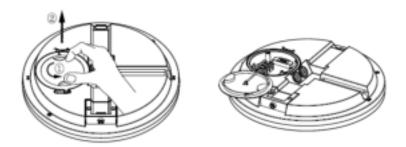
4. Secure the bracket to the ceiling.
