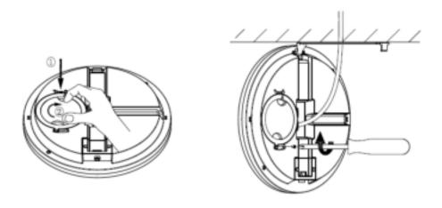
9. Push fitting into position, press until you hear the bracket lock into position .
