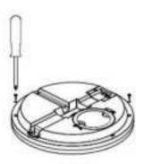
• Twist the cover anticlockwise and pull to remove it.
