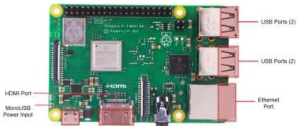
Figure 7. Raspberry Pi Model 3B+ Connections
