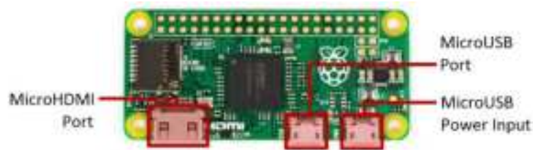
Figure 2. Raspberry Pi Zero Connections
