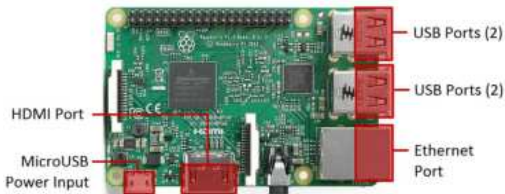
Figure 6. Raspberry Pi 3 Model B Connections
