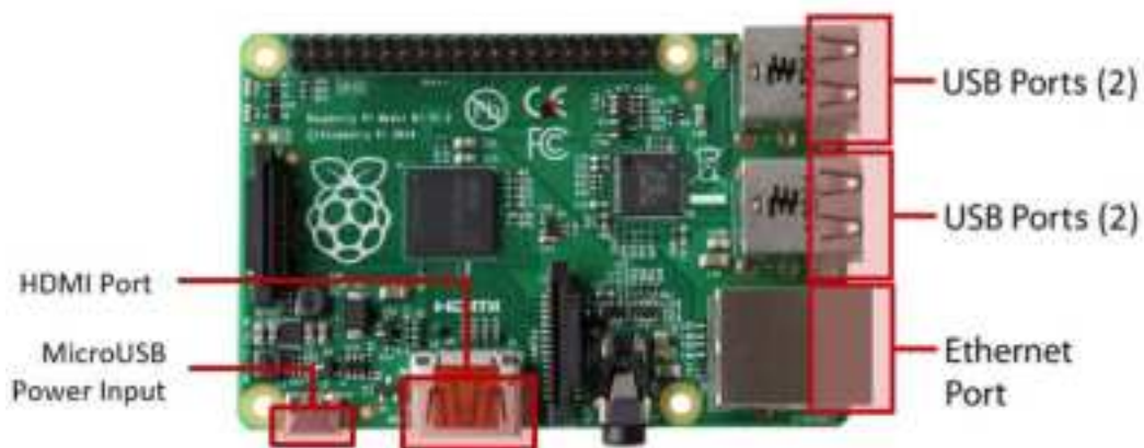
Figure 4. Raspberry Pi Model B+ Connections
