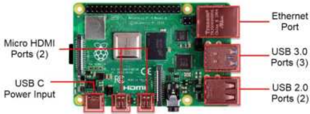
Figure 8. Raspberry Pi Model 4B Connections
