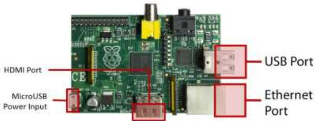
Figure 3. Raspberry Pi Model B Connections
