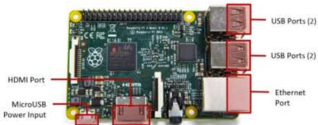
Figure 5. Raspberry Pi 2 Model B Connections
