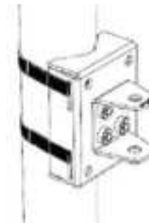
FIGURE 7 Attaching the mounting bracket to a vertical pole
