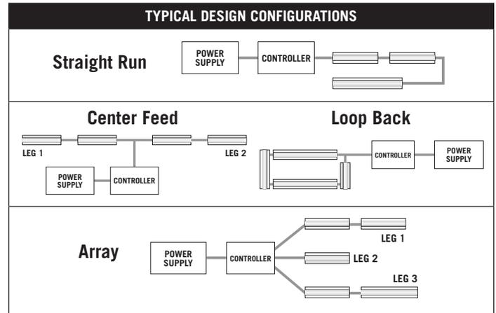
Choosing a higher wattage power supply does not necessarily mean you can run longer lengths of LED tape light. However, it will allow for more lighting legs in an array design. Exceeding the maximum lengths in the chart below will cause LEDs farthest from the power supply to appear dimmer when at 100% brightness due to voltage drop. Using a higher wattage power supply will not reduce the effect of voltage drop.
