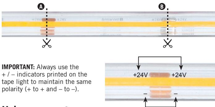
**IMPORTANT:** Always use the + / - indicators printed on the tape light to maintain the same polarity (+ to + and - to -).
