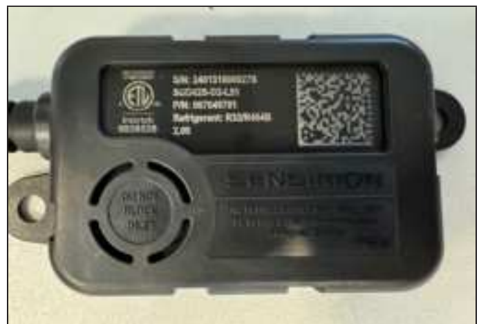
FIGURE 21. Example of Clear, Unobstructed Sensor Inlet
