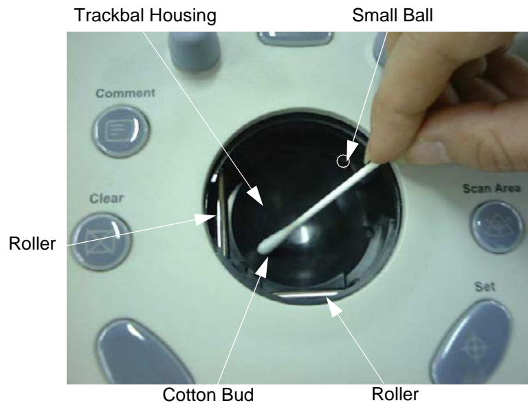
Figure 6-43 Cleaning TrackBall and Housing
