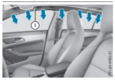
Windowbags ① are integrated in the side of the roof frame and deploy in the area from the Appillar to the C-pillar.
