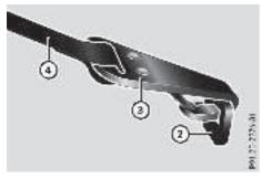
The Top Tether anchorage points are located on the rear side of the backrests on both outer rear seats.
