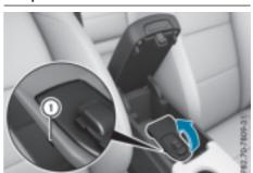
You can fold the pre-installed bracket up to improve access to the stowage space beneath it
