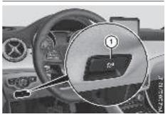
To ensure that you do not roll backwards when pulling away on an uphill slope, apply the electric parking brake.
