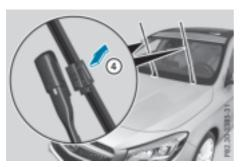
▶ Remove the wiper blade in the direction of arrow (4) away from the wiper arm.
