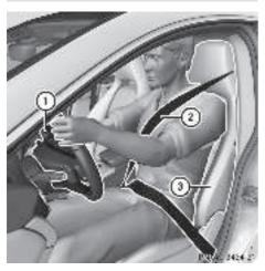
Observe the following when adjusting steering wheel (1), seat belt (2) and driver's seat (3):
