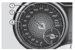
When Distance Pilot DISTRONIC PLUS is activated and there are no vehicles detected in front, one or two segments ② in the set speed range light up.
