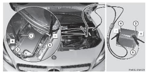
Position number (a) identifies the charged battery of the other vehicle or an equivalent jump-starting device.
