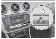
► To switch on the hazard warning lamps: press button (1).
