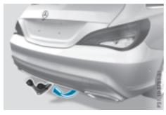
▶ Pull the ball coupling in the direction of the arrow until it engages in a vertical position. The indicator lamp on the release wheel goes out. The power socket folds down automatically. The multifunction display shows the Check trailer hitch lock display message until the ball coupling is engaged.
