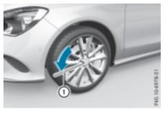
► Using wheel wrench ①, loosen the bolts on the wheel you wish to change by about one full turn. Do not unscrew the bolts completely.
