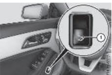
► **To open:** pull remote operating switch ① for the boot lid until the boot lid opens.
