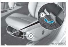
The fire extinguisher is located underneath the front of the driver's seat.
