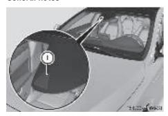
Lane Keeping Assist monitors the area in front of your vehicle by means of multifunction camera (1) attached at the top of the windscreen. Lane Keeping Assist detects lane markings on
