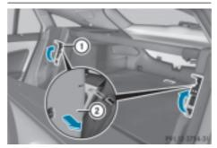
Vehicles with luggage compartment package: to enlarge the luggage compartment, you can adjust the rear seat backrests to a 15° steeper angle (cargo position).
