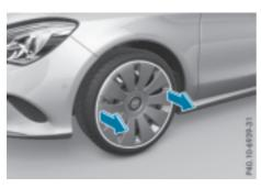
Using both hands, carefully reach into two wheel trim openings and remove the wheel trim.
