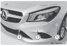
Sensors on the front bumper, left-hand side (example)
