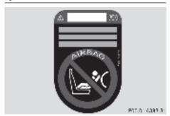
If the front-passenger seat of your vehicle is not equipped with the automatic front-passenger front airbag deactivation system, this is indicated by a special sticker. The sticker is affixed to the side of the dashboard on the front-passenger side. The sticker is visible when you open the front-passenger door.
