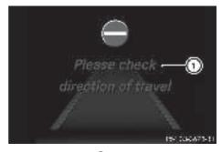
A warning message (1) is displayed in the instrument cluster if Traffic Sign Assist detects that you are passing a "no entry" sign and you are driving in the wrong direction. You will then also hear a warning tone. You should immediately check your direction of travel in order to avoid danger to yourself and other road users.
