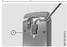
Mounting the module in the stowage compartment of the centre console
