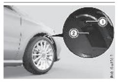
You must remove the cover in the front wheel arch before you can change the front turn signal lamp.
