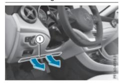
Driver's kneebag ① deploys under the steering column. The driver's kneebag is triggered together with the front airbags.
