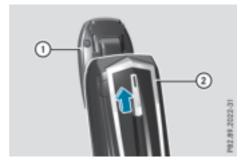
Mounting the module in the stowage compartment of the centre console
