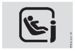
This symbol indicates an i-Size position that is suitable for attaching an i-Size child restraint system. A similar symbol can be found on the i-Size child restraint system.
