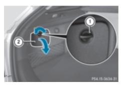
➤ To open the cover: turn handle ① anticlockwise, the fold down and remove cover ②.
