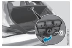
▶ Fold out hook (3) on the underside of the luggage compartment floor.
