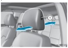
This function allows you to adjust the distance between the head restraint and the back of the head.
