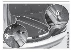
The luggage compartment cover can be stored in the stowage well underneath the luggage compartment floor.
