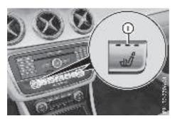
The three red indicator lamps in the button indicate the heating level you have selected.
