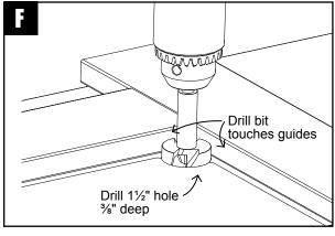
**4.** Drill a blade-start hole inside the pencil lines. With the outside edge of your jigsaw base riding on the routing guides and the inside edge supported by a <sup>3</sup>/<sub>4</sub>"-thick scrapwood block, cut just inside the lines, leaving the <sup>3</sup>/<sub>6</sub>"-wide area inside the insert-plate outline as well as the triangular areas at each corner.
