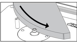
**WARNING!** Use the starting pin when routing along curved edges and only with router bits that have a guide bearing. When routing against straight edges, always use the fence.
