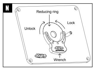
**2.** To install a reducing ring, simply drop it into the insert-plate opening and turn it by hand until it drops flush with the plate surface. Insert the pegs at the ends of the arms of the ring wrench into the mating holes in the reducing ring and rotate the ring counterclockwise **[Drawing N]**. Rotation of about % is sufficient to lock the ring in place. To remove the ring, turn the wrench clockwise and lift the ring out of the opening.
