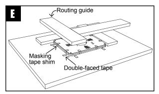
**2.** To provide clearance for installing and removing the insert plate, adhere strips of masking tape to all four edges of the plate. Then apply small pieces of double-faced tape to one face. (Use just enough tape to keep the plate in place. Too much tape will make the plate hard to remove later.) Reposition the insert plate on your router table top and firmly press it into place.
